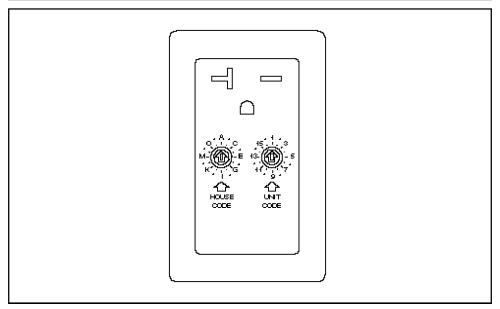
The Heavy Duty Appliance Module is designed to handle 20Amp/220V loads to control air conditioning, water heaters etc.
