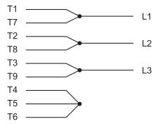
For 230V, Single Phase, Wiring (model MVP<sub>Liquid</sub>1PH): Bridge the wires as shown. Then, connect L1 to P1 and L2 to T4/T5.
