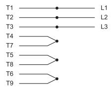
4. For 230V, 3 Phase, Wiring (model MVP<sub>Liquid</sub>3PH): Bridge the wires as shown. Then, connect L1 to T1/T7, L2 to T2/T8, and L3 to T3/T9.
