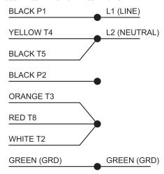
For 115V, Single Phase, Wiring (model MVP<sub>Liquid</sub>1PH): Bridge the wires as shown. Then, connect L1 to P1 and L2 to T2/T4/T5.
