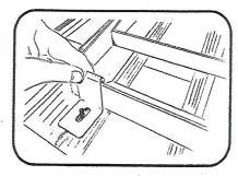
Slide bolts into groves on slat and place hook plate over edge of holder.
