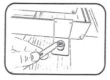
Tighten with 13mm spanner,wrench.
