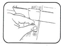
Thread on nyloc nut onto bolts.
