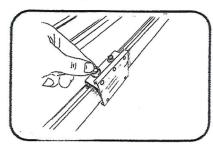
After sliding to position required tighten with 10mm spanner wrench.
