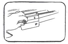
Close cover and tighten with thumb lock.
