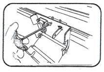
Fasten axe bracket to K9 mounting kit with bolts provided.
