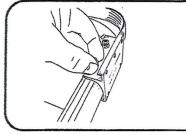
Place K9 mounting kit onto side rail and turn bolts to align with slot.
