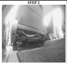
Passenger seat. Feed 2 front and 2 side webbing straps underneath the seat and tie to the buckles at the back of the seat.
