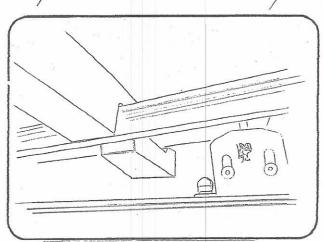
Shower arm should sit over edge of rack and under slat on the sides and load bar at the back.
