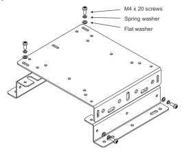
The supplied step-plates can be used to raise the NLDC-25 above obstructions such as pipes or cables if necessary.
