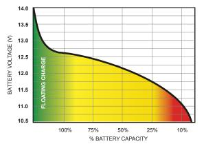
Voltages measured above 12.6V on the battery indicate that the battery is charging or may have a *"floating charge".* The Dual Battery Controller follows the battery discharge curve and gives a good estimate of battery capacity based on voltage.
