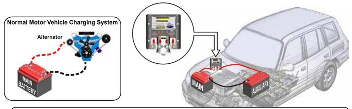
DO NOT RELY ON THE VEHICLE'S BODY TO PROVIDE A NEGATIVE ELECTRICAL EARTH PATH
