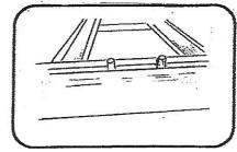
Slide 6mm bolts into rail and centralise between table slides.
