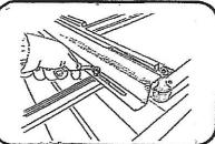
Thread nyloc nuts onto bolts secure with 13mm spanner/wrench.
