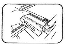
Slot bolts into slide rails and place table slide into position.
