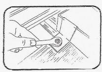
Tighten with 13mm spanner wrench.
