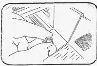
Thread on nyloc nut onto bolts.
