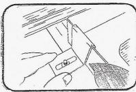
Once holder is in place on the rack place hook plate over the edge of holder.
