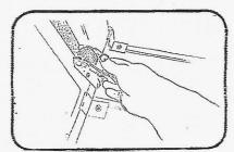
Fasten the ratchet by cranking the handle In order to secure water tank.
