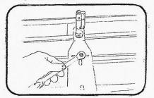
Tighten with 13mm spanner wrench.
