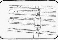
Do the same with the front K9 barcket but leave the bolts loose so as it can slide.
