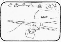
Place the Max Trax onto K9 brackets and slide front K9 bracket so as holes a line. Secure with 13mm spanner wrench.
