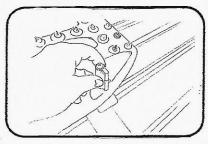
Turn Max Trax Pins in order to secure Max Trax to K9 bracket it.
