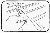
Place K9 bracket on rack and thread on nyloc nut onto bolts.
