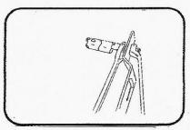
Secure with 17mm and 22mm spanner wrench
