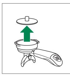
Remove the filter holder, take out the blind filter disk
