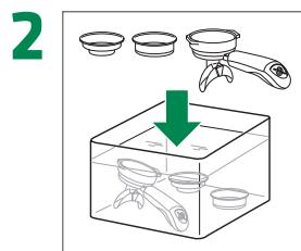
Immerse filter holder/unlocked filter in solution for at least 20 min.
