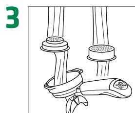
Rinse filter holder/filter thoroughly under running water
