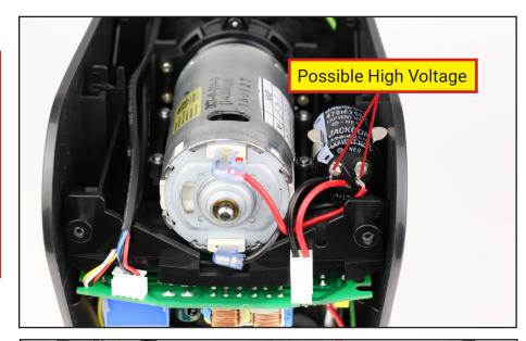
Unplug display, power cord and motor from circuit board
