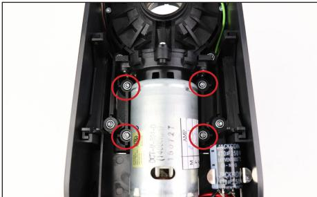
Remove the 4 screws securing the power board bracket.
