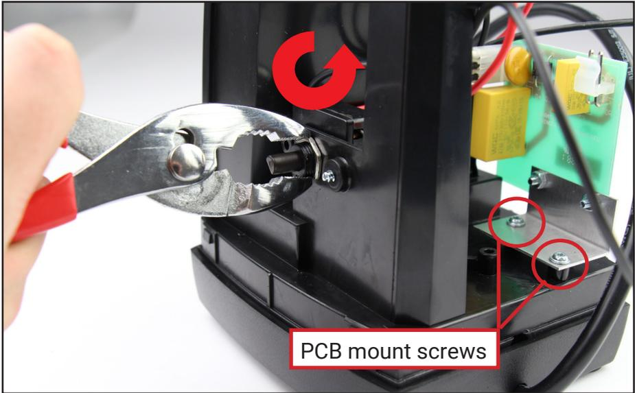
Remove the screw which mounts the switch to the chassis. The switch should come free easily.
