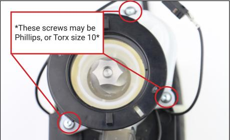
Unplug the motor and lift the gearbox/motor assembly from the chassis.
