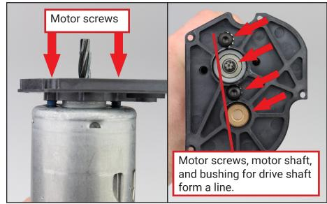
Install the motor/motor plate into the gearbox housing.
