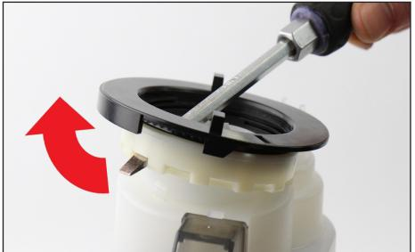
Lift the adjustment ring off, taking care to secure the spring-loaded detent.
