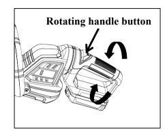
**Note:** The trimmer will only operate at one of these locked positions. The handle is locked when the rotating handle button is securely in place and the handle will no longer move to either side
