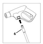
5. **Install the high pressure pipe to the main body.** Push the high pressure pipe to the outlet connector, tighten it by rotating the pipe connector clockwise.
