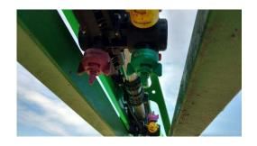
nozzles those speed changes can result in variable pressures and different spray qualities, along with possibly having to change nozzle selection for each field. The Duo React System from Hypro, supported by AgStar addresses the applicator's need for operational flexibility and consistent spray quality combined with the use of air induction nozzles for overall superior spray performance.
