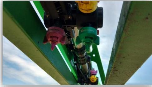
The Duo React utilizes a "DUO" nozzle body with a primary position (single) and a secondary (quad) turret position. The system can switch from primary to secondary nozzles instantly at a programmed setpoint, as well as spraying with both nozzles A+B at the same time. The operator can also manually select the nozzle(s) in operation allowing for total operator control when desired.
