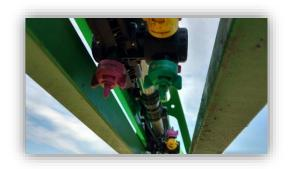
spray quality, forcing the operator to under/overdrive the unit or use up valuable time changing nozzles manually. The Duo React System from Hypro, supported by Nozzle Ninja addresses the applicator's need for operational flexibility and consistent spray quality combined with the use of air induction nozzles for overall superior spray performance and drift control.
