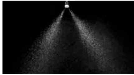
Sturdy twin 30° incline/decline patterns provide superior canopy penetration through pattern integrity.
