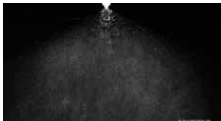
Low pressure performance allows for complete pattern formation and even coverage down to 15 psi (1 BAR).
