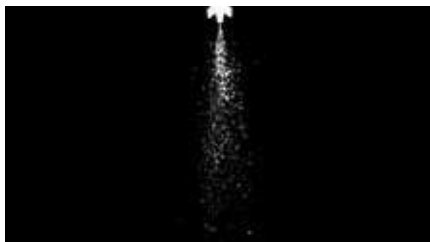
Straight through design squeezes fluid flow to create the spray pattern versus deflecting fluid flow and creating un-needed spray drift.
