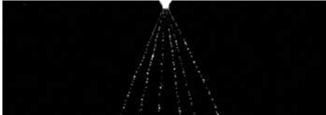
110° wide pattern consisting of 6 equally spaced streams providing uniform deposition of liquid fertilizers. Each individual stream was engineered to hold stream integrity and not break apart to avoid unwanted fertilizer burn on post emerge applications.
