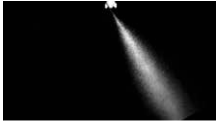
Inclined 30° spray pattern of medium to fine droplets provides superior coverage and canopy penetration.
