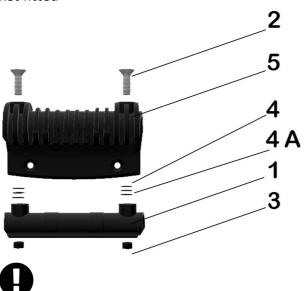
It is not recommended to remove bracket (5) from the gear bag unless it is damaged and requires replacing. The wheels on you bag can also be replaced if damaged.
