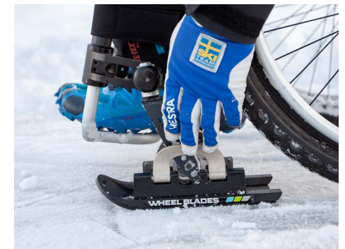
4. Close the quick-release astener and off you go.
