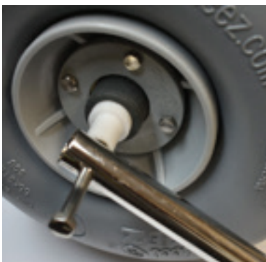
Center wheel between caster forks and install bolt
