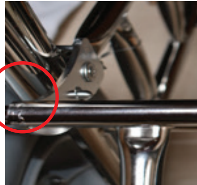
Locking bar and pin engaged.
