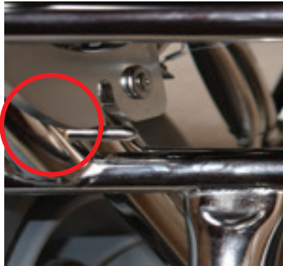
Locking bar and pin disengaged.
