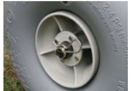
Reinstall Hitch Pin to retain wheels.
