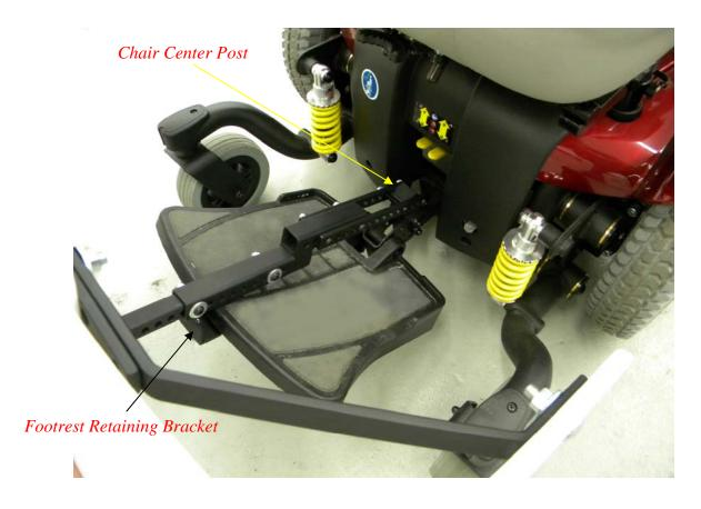
**2.** With the footrest tilted down, the footrest retaining bracket should be fully hooked on the bottom of the footrest. Tighten the center post mounting strap bolts.
