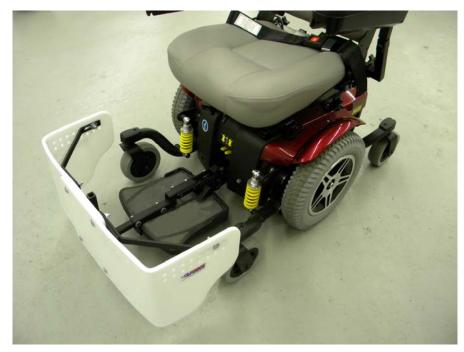
**3.** With the footrest tilted down, tighten the footrest retaining bracket bolt.
