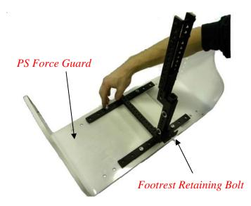
**5.** Attach the receiver assembly to the PS Force guard as shown (*left*).
