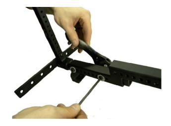
**4.** Determine the center post width on your specific chair and fasten the mount straps to the receiver assembly with (2) 1-3/4" or (2) 2" button head screws as shown (*right*).
