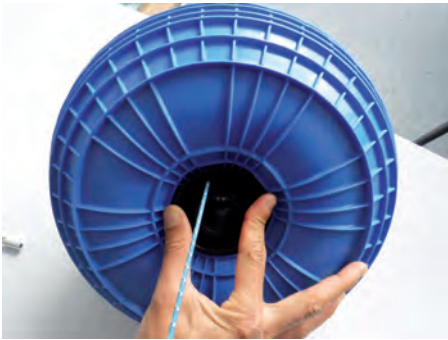
Check the hub is properly inserted to the stop and the cord does not block the axis.
