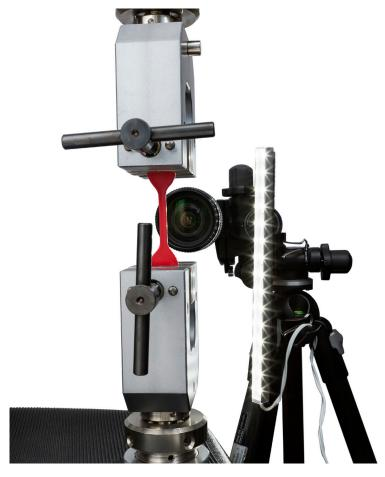
The VE1 video extensometer is a high precision instrument that uses a non-contacting optical measurement system based on a digital camera and real time image processing to measure the longitudinal and transversal strain during a tensile test. The system measures longitudinal strain between two applied lines at a rate of up to 100 Hz. The strain data is synchronized and transfered to NEXYGENPlus 3 software (Series Plus & LS machine). An optional analog signal can be used for older machines.
