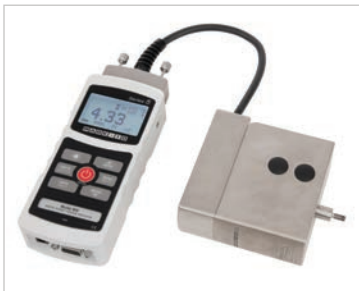
FS05 force sensor connected to an M5I indicator via AC1083 adapter for off-site calibration
