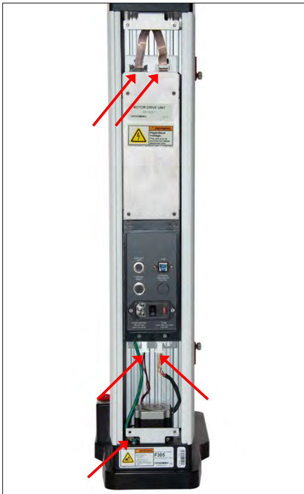
Locations of connectors, ground wire, and bracket
