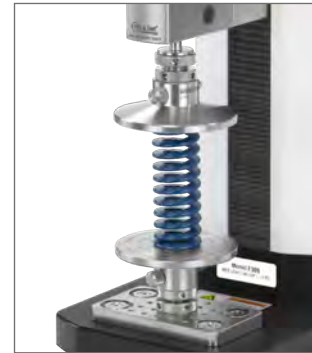
Compression spring testing
