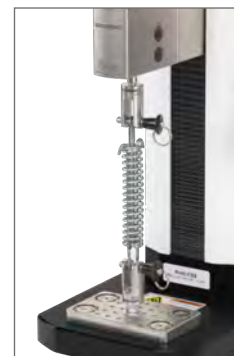
Tension spring testing
