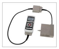
AC1084 Plug & Test<sup>®</sup> Extension cable 24 in. / 610 mm extension facilitates easier connection to a Model M5I or M7I indicator for calibration.
