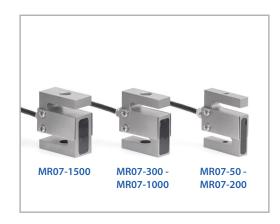
Series R07 force sensors measure tension and compression force, and are designed for use with Models F755, F755S, F1505, and F1505S test frames. Capacities available from 50 to 1,500 lbF [250 N to 7.5 kN]. Also compatible with Mark-10 indicators (sold separately) through unique Plug & Test® technology. Includes a certificate of calibration with data.
