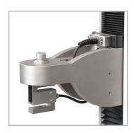
Series R07 sensor is shown mounted to the crosshead of an F1505 test frame.
