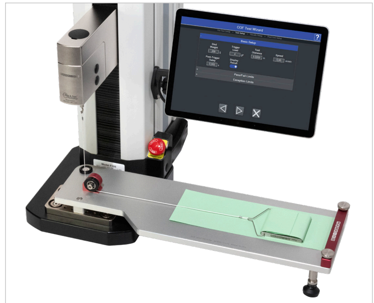
An F305-IMT advanced test frame configured with a G1086 coefficient of friction fixture.
