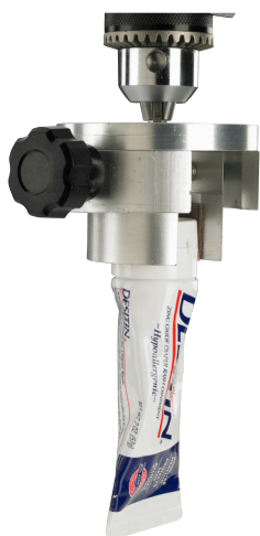
STS sensor attached to the B200308 torque fixture for measuring cap torque strength.
