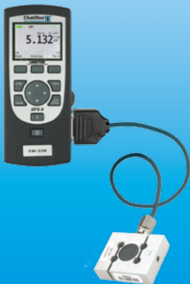
SLC Sensor attached to the DFS II-R-ND gauge.
