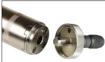
Fig. 10.1 The attachment and main sensor body mate with a pin and threaded ring.
