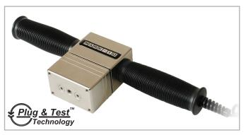
Series R05 fully enclosed smart sensors are designed for pull / push measurements. Useful in ergonomics testing, workplace safety testing, and general lifting or tension / compression requirements. Threaded holes are supplied to accommodate various mounting configurations and attachments. For up to 500 lbF [2,500 N].
