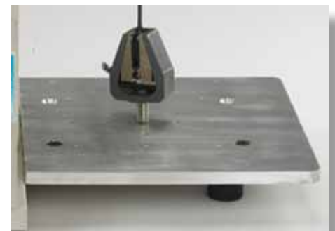
Shown: An optional extended work table fits onto the T-Slot. Pre-drilled holes make fitting fixtures and specialized testing jigs easy.
