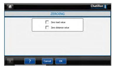
Select "ZERO LOAD VALUE" and / or "ZERO DISTANCE VALUE" as required. Note that the crosshead will stop briefly to allow the system to zero.
