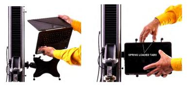
Once fitted, position the Laptop console where it can be easily viewed and operated by the user. Once you have positioned the Laptop console, tighten the hand screw so that the Laptop console is secured in the intended position. Ensure that the control console does not move when pressing on the touch screen.
