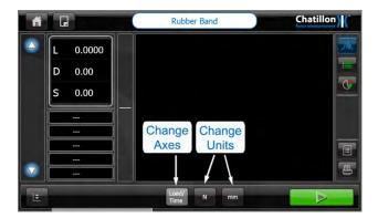
Therefore, pressing the "CHANGE AXES" button changes the graph to show Distance / Time as shown below.
