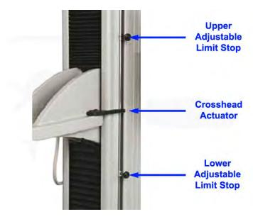
If during a test or when maneuvering the crosshead, a limit stop switch is activated, an error message will be displayed on the control console.
