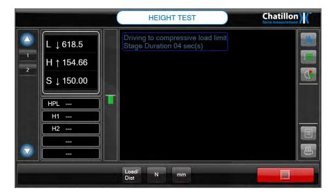
Note that the "Live" display on the left-hand side of the "Graph" area shows the "Height" during the test, e.g. 154.66mm in the example screen shown above.
