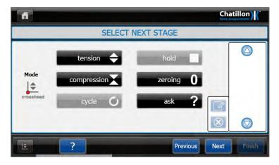
The Icon at the left-hand side of the screen shown above shows "Height Mode" (Red dot at the bottom of the vertical line).
