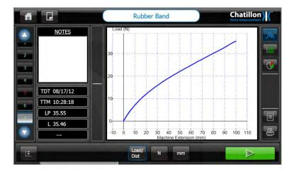
The screen shown above indicates that 7 samples have been tested. This screen also shows that sample number 5 failed the pass/fail criteria because numbering on the button marked "5" is shown in red.
