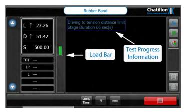
The vertical "Load Bar" indicates the actual load on the Loadcell and will be displayed as a small horizontal line when there is no eye end or grip fitted to the Loadcell.
