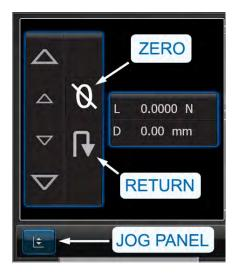
The new crosshead position can also be manually zeroed using this Panel.
