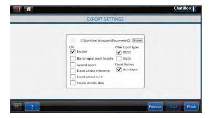
After the Test results have been selected in the "**RESULTS**" screen, the RS232 output will export results as the example below:
