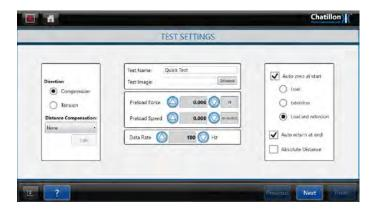
Select the required "**Direction**" using the controls on the left-hand side of the screen. Note that Compression means move the crosshead downwards during the test and Tension means move the crosshead upwards during the test.
