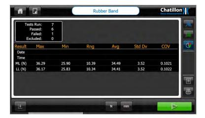
The test statistics are shown above. The top left area shows the test status for every test. The test status is normally the pass/fail status and the example screen shows that 7 samples were tested and that 6 samples passed and 1 sample failed.
