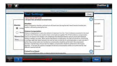
The first configuration screen displays the "Basic Settings" for the test and includes "Direction", "Distance Compensation", "Preload", "Data Rate", "Auto Zero" and Auto Return".
