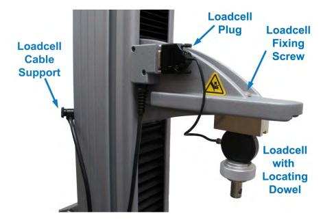
The Loadcell Cable Support can be adjusted up or down the Column Extrusion by loosening the thumbscrew. Ensure there is plenty of length in the cable connected to the crosshead so that the crosshead can travel without pulling on the cable.
