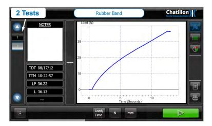
The left-hand vertical area of the screen now displays two buttons, marked "1" and "2", to show that 2 tests have been performed. Both numbers are shown in green because the measured values are within the optional pass/fail parameters. A number will be shown in red if the relevant test fails the pass/fail parameters.
