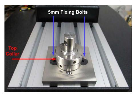
The top collar on the Lower Anchor Pin should be used to secure the lower grip in place. Use the small spanner wrench provided to tighten the collar upwards against the bottom of the lower grip.
