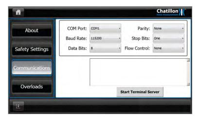
Set the communication parameters as shown in the above picture (as listed below) Baud Rate = 115,200
