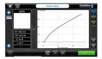
The picture above shows the default graph axes of Load / Time.
