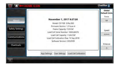
This central area shows the Current Date and Time, Force Tester Type, Force Tester Serial Number, Force Tester Firmware Version, Frame Capacity, Loadcell Serial Number, Loadcell Capacity, Last Loadcell Calibration Date and Console Software Version.
