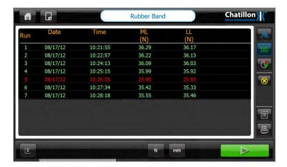
The data table shown above displays the measured results for every test. The values are displayed in either red or green depending upon the pass/fail criteria for each test.
