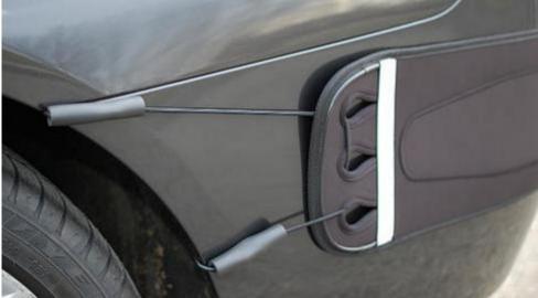
**STEP 8b** – Our "Super Strong Suction Cups" require a relatively flat surface for proper adherence. Make sure the area of your car (fender area) is appropriately flat by testing a suction cup on the general area where they will be installed. Make sure this area is extremely clean for best adherence.
