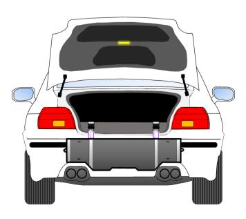
STEP 7 – Once you have confirmed the "Main Center Body" is properly centered on your bumper and hanging at the height chosen for your vehicle's installation, <u>approximate</u> the positioning of one "Side Piece" and <u>temporarily</u> attach it to the under-side of the "Main Center Body" aligning the top and bottom border edges so that the side piece is straight and parallel with the "Main Center Body's" top and bottom edges (your vehicles trunk can be open or closed during this procedure).
