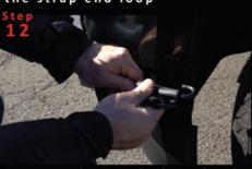
Temporarily attach the S-hooks to the inside edge of the wheel well
