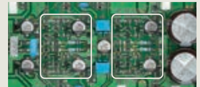
2-parallel circuit layout of MCS+ principle
