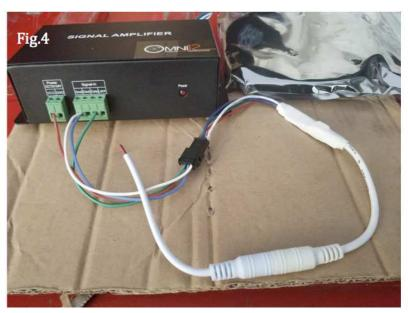
**Step 4:**There are 8 outlets on the Signal Out end of the signal amplifier. Connect the hardwired ends of 4 included extension cables. As shown in Fig.5 to outlets 1-4 of the signal amplifier.
