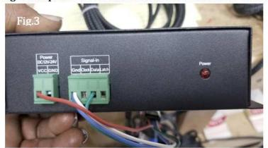
damage. Connect the hardwired plug ends from the remote controller (Model #: Y-99-1010) to the Signal In of the included signal amplifier (Model #: Y-99-1012). Connect the red wire to the VCC 12v terminal. Connect blue and white wires to the 4 inlet Gnd terminal on the signal
