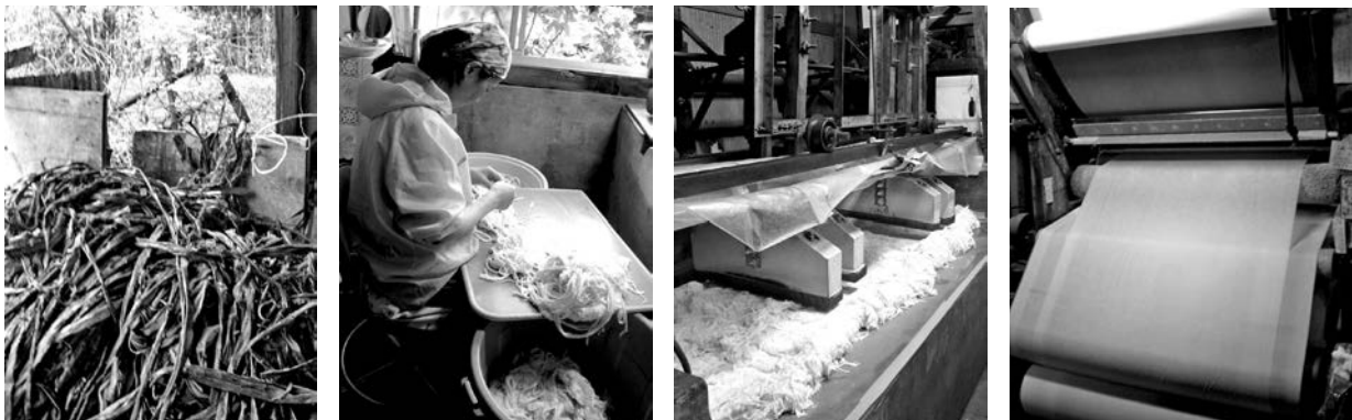
(Left to right) Steps for making machinemade washi at a typical paper mill: Kozo fibers being cooked, the chiritori process, beating the fibers, and roll production.
