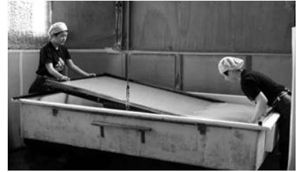
Iwano's large handmade papers require teams of at least two people for the nagashizuki method of sheet forming.
