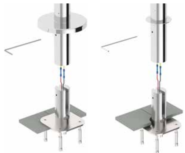
Over Tile Installation
