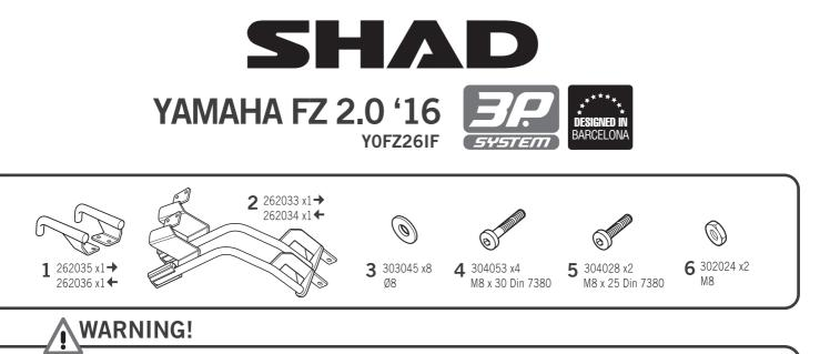
**GB** Do not fully tighten the screws until it is ensured that the KIT is correctly attached and aligned.
