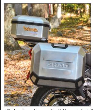
The bags themselves were formidable; created out of 100% forged aluminum alloy. These aerodynamic bags are stronger and lighter than those of their competitors and features a reduced cross-section of 1.2mm to give them minimum weight with maximum resistance. After the install was complete the rock-like solidity of these mounted bags was impressive.
