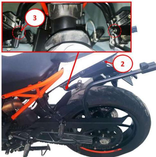
Remove the handle pillion from motorbike then install the 3P kits and replace the original bolts with parts no.2
