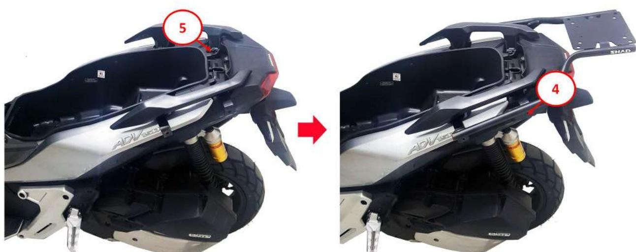
Install the fitting kits in to motorbike by using part no.4
