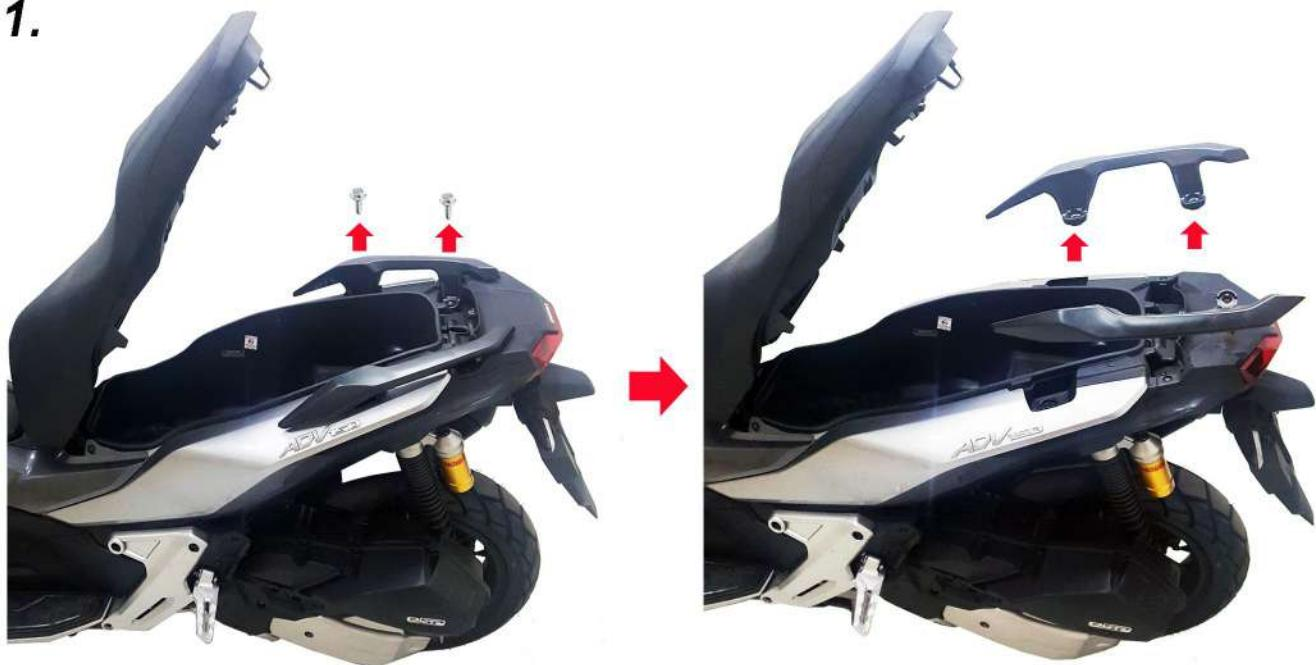
Open the handle pillion of motorbike by dissassembly original bolts
