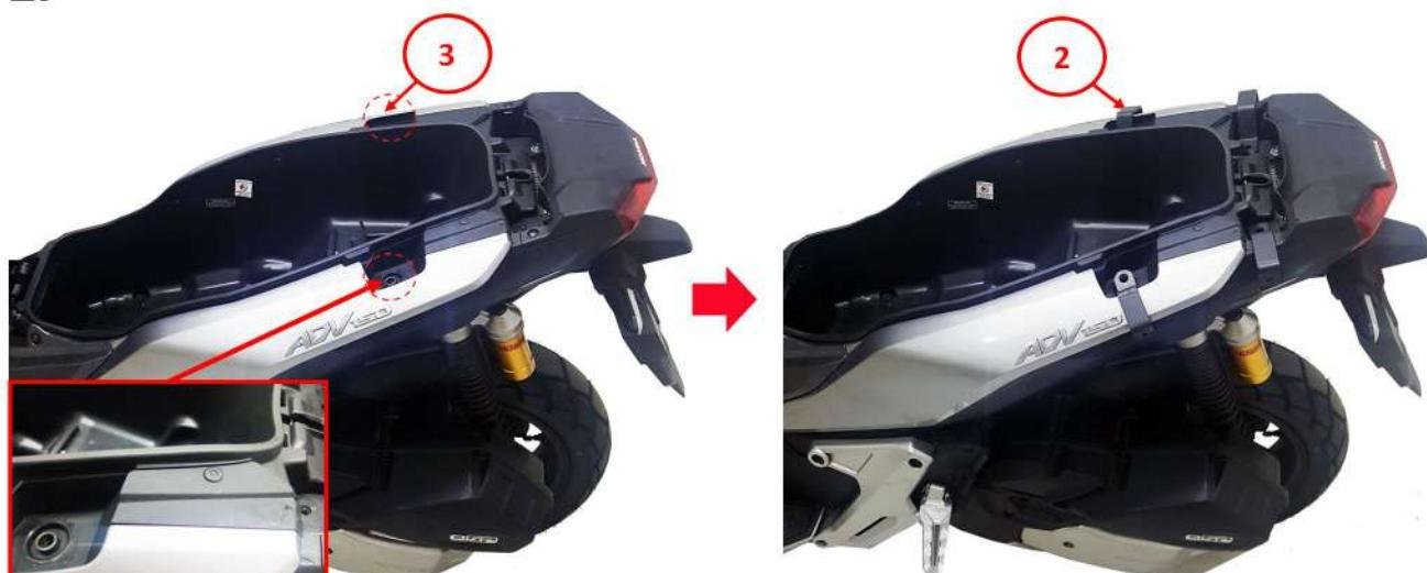
Put part no.3 in to motorbike then Assembly part no.2 ( short metal part in front and long metal part in rear )by using part no.5
